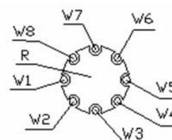
Working electrodes are marked anticlockwise as standard
