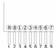
Contacts numbering begins from the left corresponding working electrode number is in circle
