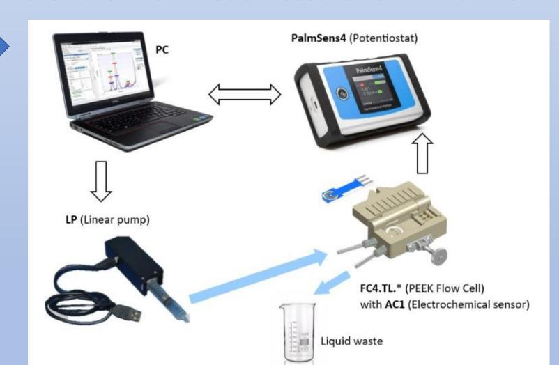
The GOD sensor works best in flow mode. For these purposes, we recommend the use of flow **cells FC2 or FC4** in conjunction with a suitable **pump**.
