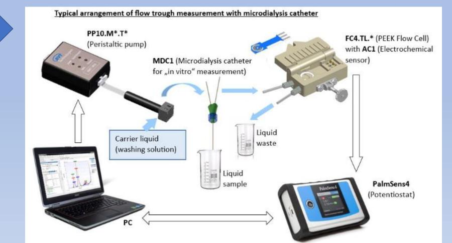
Combination of flow mode measurement using flow cell **FC\*** in connection with mycrodialysis catheter **MDC1**.
