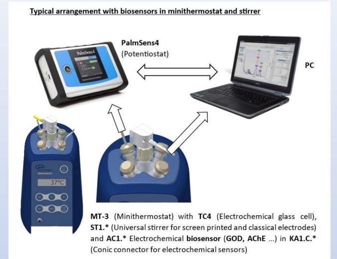
The GOD sensor can be inserted into the **KA1.C** connector and then inserted into the glass electrochemical cell **TC6 or TC7**.
