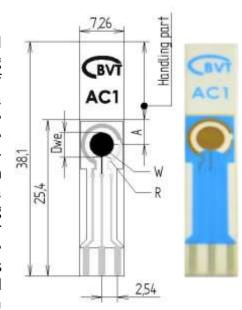
The handling part can be broken off and sensor can be inserted in the standard BVT flow cells.
