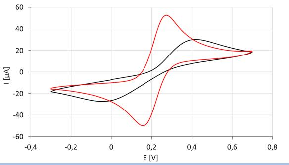
**BVT offers \*unactivated versions of both graphite sensors** W4 and W5 for standard tests and direct measuring. For specialised testing and more precise results **it is recommended to have the W4 and W5 activated** – see graph. (the activation in most cases, is unique for each type of test being carried out).
