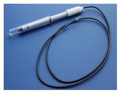
used measuring apparatus, with internal resistance of above 10<sup>9</sup> - 10<sup>12</sup>. Standard electrical connecting cable is 0.8 to 1 m. coaxial cable with BNC connector. The work with ion selective electrodes is time effective, requires an only small amount of chemicals, and a friendly price of measuring equipment MPH472.
