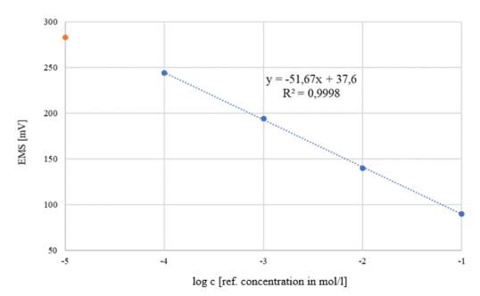
A 15-channel potentiostat from the monokrystaly company was used for potentiometric measurement. KCl samples with a concentration of  $10^{-1}$  to  $10^{-5}$  mol/l were diluted with distilled water)
