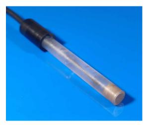
Electrodes are applicable to all commonly used measuring apparatus, with input resistance of at least  $10^{12} \Omega$ . The work with ion selective electrodes is time effective, requires an only small amount of chemicals, and a friendly price of measuring equipment (potentiostat with measuring method potentiometry).
