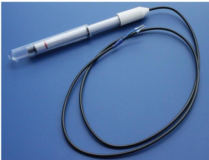
used measuring apparatus, with internal resistance of above  $10^9$  -  $10^{12}$ . Standard electrical connecting cable is 0.8 to 1 m. coaxial cable with BNC connector. The work with ion selective electrodes is time effective, requires an only small amount of chemicals, and a friendly price of measuring equipment MPH471.
