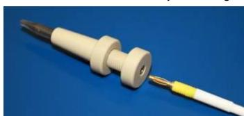
electrode itself is polyethylene tip profiled with paste. The graphite paste is delivered as a standard electrode. Standard connection is with a 2 mm banana plug. Paste electrode (PEc) is designed for measurements with TC4, TC5 and TC6 glass cell. PEc is used for
