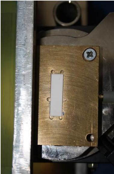
**Fig.6.10** Insert substrate in the holder (The ceramic substrate for AC1 sensor on fig)
