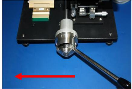
**Fig. 6.2** – of screen from printing position (red arrow)-movement of screen to left position
