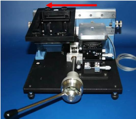
**Fig. 6.3** The screen holder is in left position prepared for screen insertion
